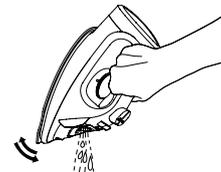
9. To prevent corrosion of the soleplate vents, plug the power plug into a socket-outlet, stand the iron up, set the temperature select indicator to "MAX" and preheat for about 5 minutes.
