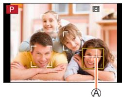
**Changing the eye to be in focus****Touch the eye to be used for focusing**
