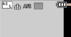
**Remaining battery** (only when using battery)
