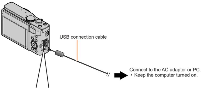
**When charging the camera, connect the USB connection cable to the [USB/CHARGE] socket.**
