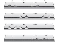
There is a problem with this unit. Disconnect the AC power supply cord from the AC outlet, reconnect it to the AC outlet after about 30 seconds. If the problem still persists, disconnect the AC power supply cord and consult your dealer.
