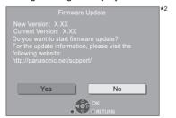
Select "Yes" to start downloading the firmware. When the firmware update starts after the downloading is finished, a black screen is displayed and the POWER LED flashes rapidly.
