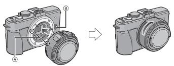
• Do not press the lens release button (B) when you attach a lens.
